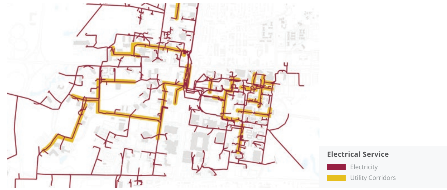
The maroon lines illustrated above indicate the paths of electrical service on campus. The yellow areas highlight utility corridors where chilled water, heating hot water, and electrical service are coincident. Impinging on these corridors would require significant financial investments to move utility lines.
