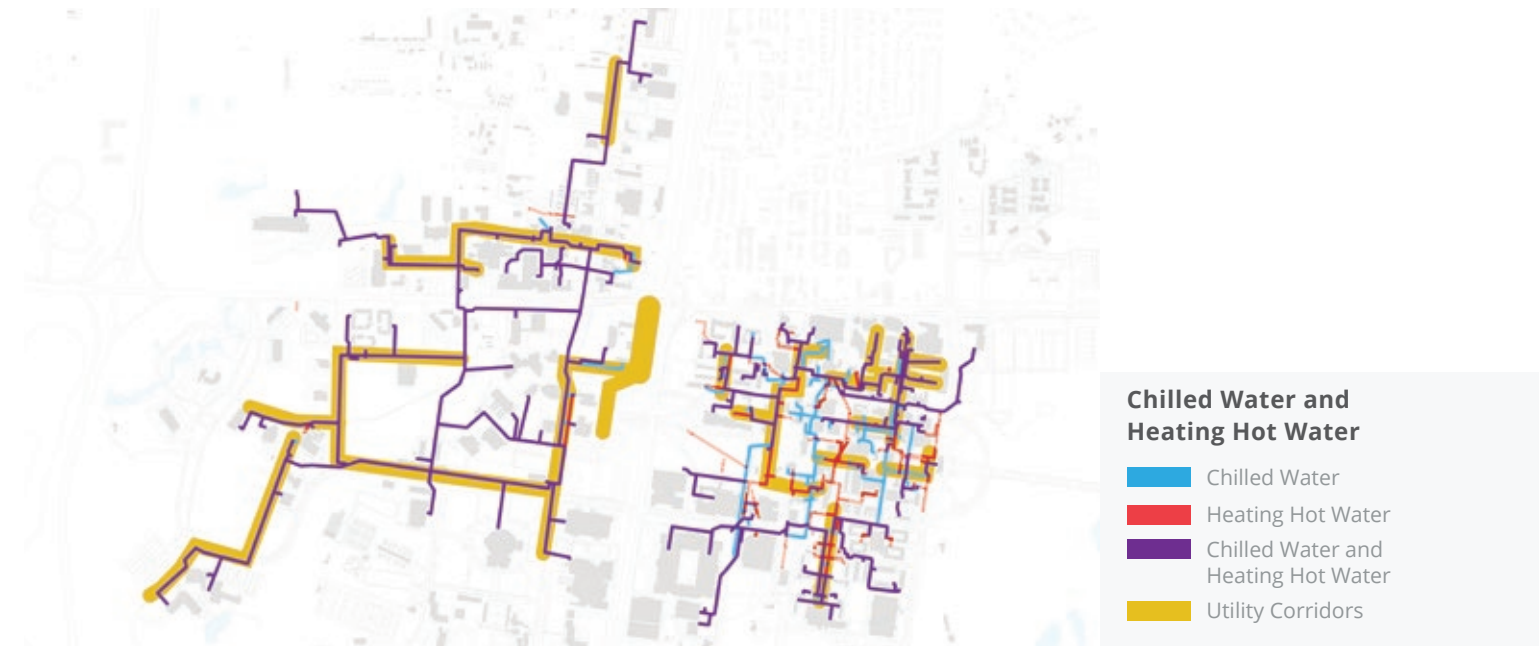
The purple lines illustrated above indicate where the paths of chilled water and heating hot water are coincident. The yellow areas highlight utility corridors where chilled water, heating hot water, and electrical service are coincident. Impinging on these corridors would require significant financial investments to move utility lines.
