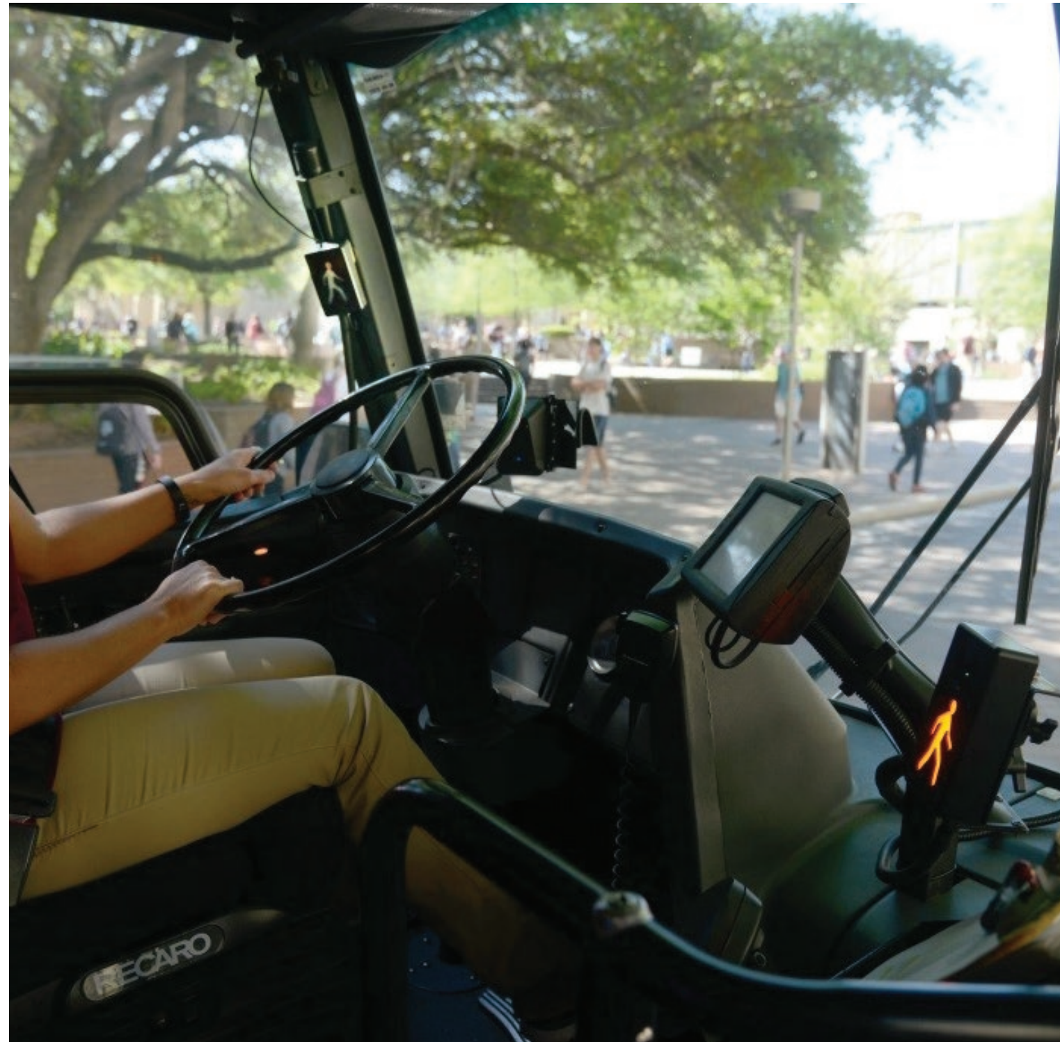
Texas A&M Bus Piloting Collision Avoidance System
